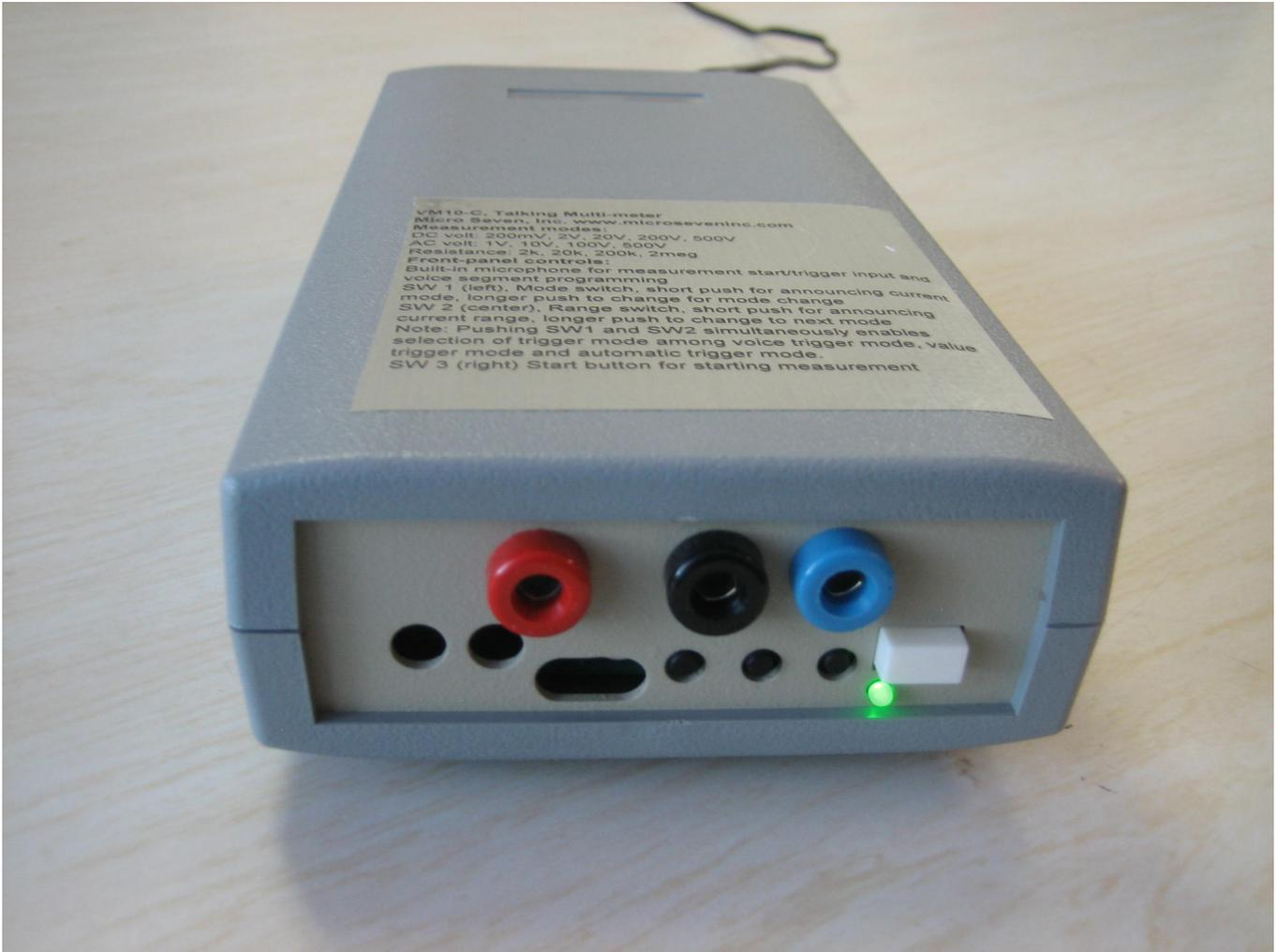
MICRO SEVEN-Model VM10a, Scope-Meter, oscilloscope/Talking Digital Multi-meter is shown in above picture. The rear view of VM10a is shown below.
